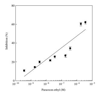
**Figure 1.** Calibration curve between inhibitor concentration and %I plotted in semi-logarithmic scale. Five values of frequency shift at adjacent measuring time were determined and error bars were inserted.
